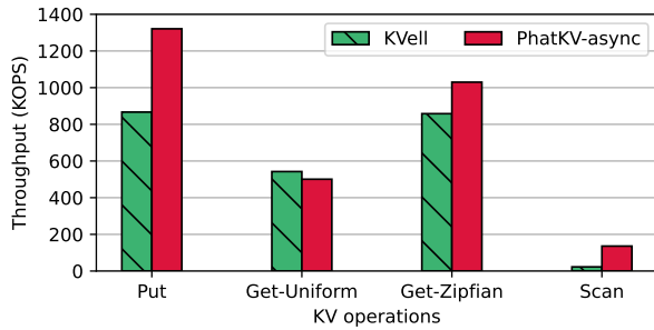
Fig. 12. Micro-benchmark results of KVell. This figure shows the throughput comparison between KVell and PhatKV-async.
